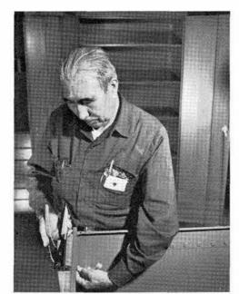
COST SAVINGS of about \$1000 a year are realized because of an innovation suggested by Jose Valdez (4575). He proposed that hand-held mechanical rivet guns be used to assemble office supply cabinets instead of a bolt, washer, and nut assembly. The rivets provide a tighter clamp in addition to savings of time. The Cost Improvement Policy Committee commended Jose for the time-saving suggestion.
